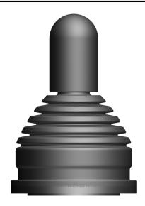
This joystick type is based on our well known SK60 joystick and equipped with Hall Effect sensors. An almost non-existent installation depth makes it possible to mount the joystick directly onto the panel while its two axes allow a full deflection of 20° in every position.
